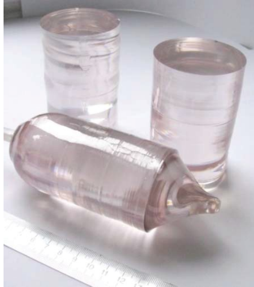
ZnWO 4 crystals for nuclear physics and medical radiography grown by Cz method
