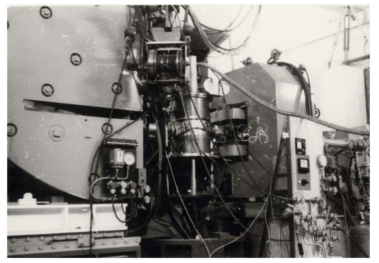
$\gamma \ d \to \pi^0 \ d$  radiator, magnet, liquid  $D_2$  target, spectrometer, 2 scintillators scalers, pulse-height analyser (paper output), no computer  $\Rightarrow$  tremendous opportunity to learn the experimental trade
