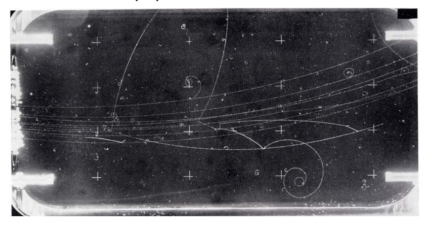
Picture taken with the BP3 bubble chamber (on display in front of Bat. 208), built by A. Lagarrigue and exposed to a pion beam at Saturne (Saclay)
