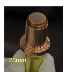
Grain Size ~ 0.3- 0.5 mm **Roughness: Ra ~3 nm; PV= 15 nm (bfr) Roughness: Ra ~ 8 nm; PV= 110 nm (aftr)** Diamond Tool Waviness: 0.1 mm
