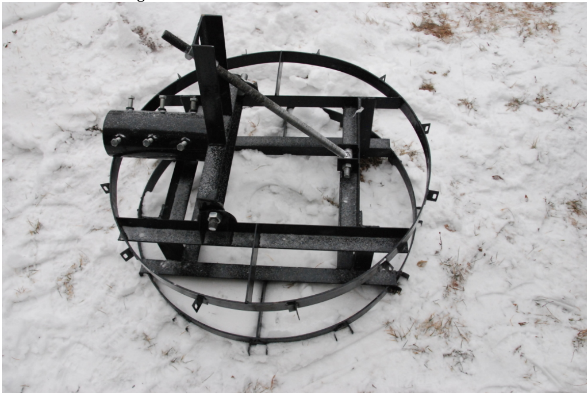
Rectangular shape made from angle is the core of the mount. Rolled steel rings create attachment points for the dish and struts.
