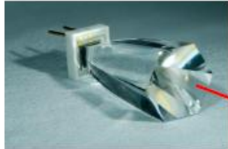
MPPC S10362-33-50C coupled to a cone light concentrator
