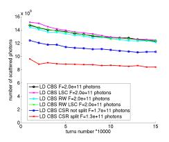
Compton backscattering flux for different beam dynamics effects. In the case of the CSR simulations, if the beam did not split 97% of the particle survived (blue) and 50% survived in the case the beam did split (red). F is the total flux integrated over 150000 turns.
