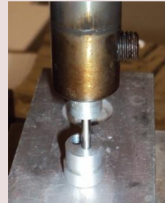
Pressing to compact the powder
