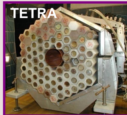
3He neutron detector (Dubna-Orsay collaboration)
