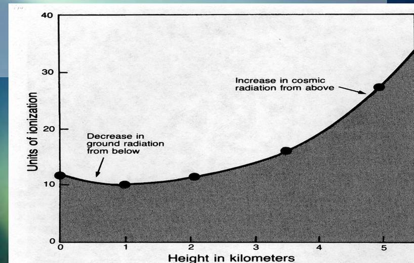
Readings on ionization chamber Victor Hess carried aloft in the Böhmen. Above four kilometers the ionization rose rapidly indicating "that rays of very great penetrating power are entering our atmosphere from above". These cosmic rays contain the only modern samples of matter from outside our solar system which can be investigated directly.
