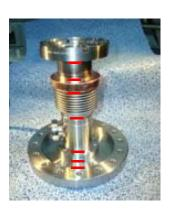
2<sup>nd</sup> step: copper plating of the assembled parts:
