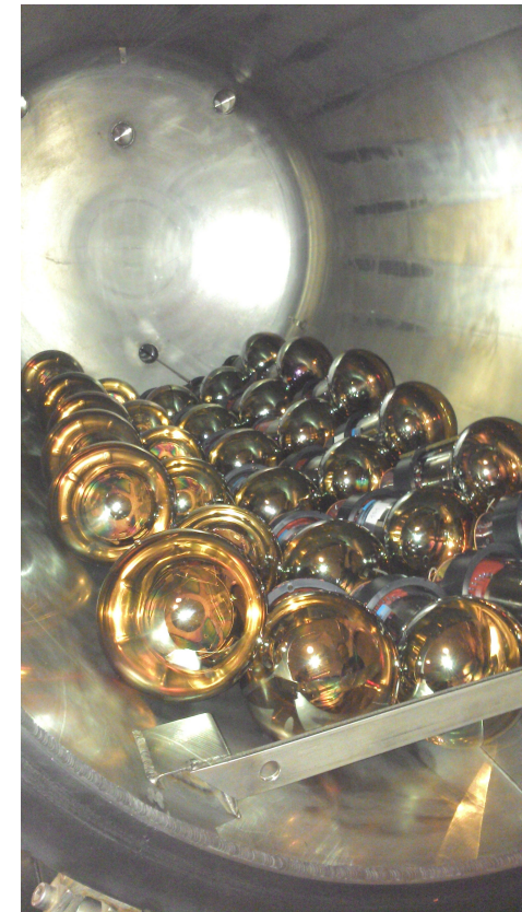
5" PMT from NEMO-3 ( N = 30 ) A_{\text{em}}(^{222}\text{Rn}) < 119 \mu\text{Bq}/\text{PMT}
