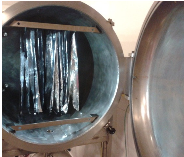
Aluminized Mylar ( 36 \text{ m}^2 ) A_{\text{em}}(^{222}\text{Rn}) < 97 \mu\text{Bq}/\text{m}^2
