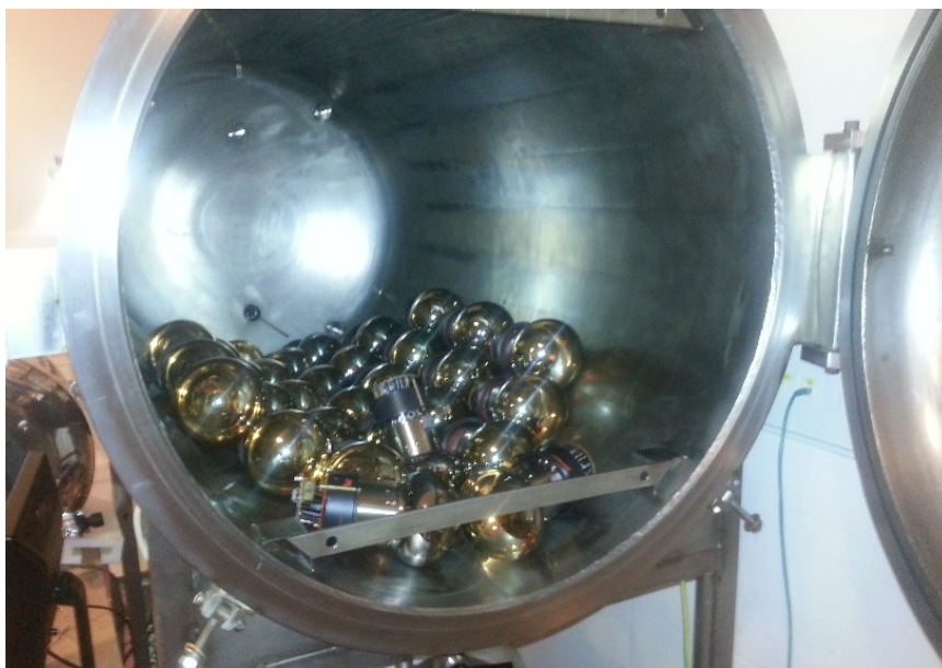
Large emanation tank – 0.13 mBq/m 2 (for 30 m 2 sample)
