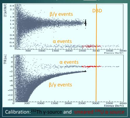
First bolometric measurement of 2vββ of <sup>100</sup>Mo with a ZnMoO<sub>4</sub> crystal array
