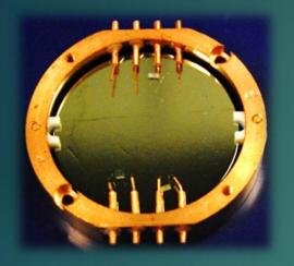
To allow proper calibration of the LD a <sup>55</sup>Fe source, producing two X-rays at 5.9 and 6.5 keV, is used
