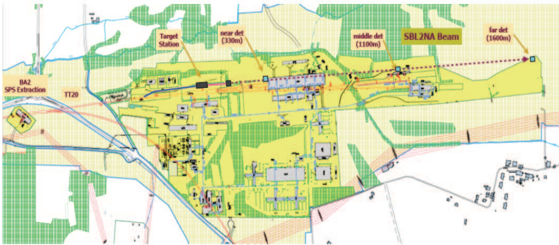
Figure 139. The new SPS North Area neutrino beam layout. Main parameters are: primary beam: 100 GeV; fast extracted from SPS; target station next to TCC2, \sim 11 m underground; decay pipe: 100 m, 3 m diameter; beam dump: 15 m of Fe with graphite core, followed by muon stations; neutrino beam angle: pointing upwards; at \sim 3 m in the far detector \sim 5 mrad slope.
