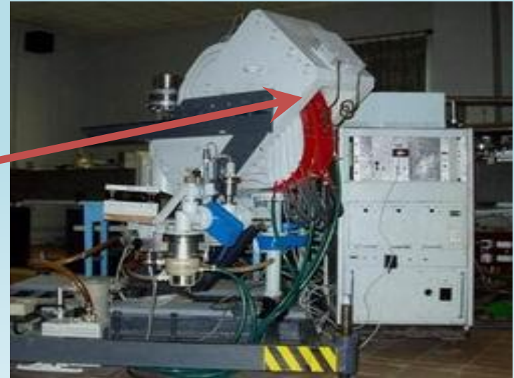
Magnetic spectrometer with double focusing ( \Delta E/E=3,2 \times 10^{-3} )
