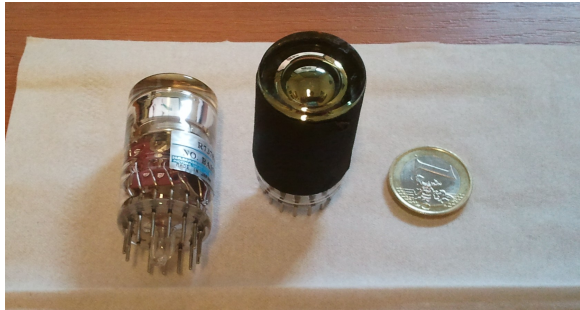
HAMAMATSU PMT (R7378A) with radiation hard fused silica incoming window
