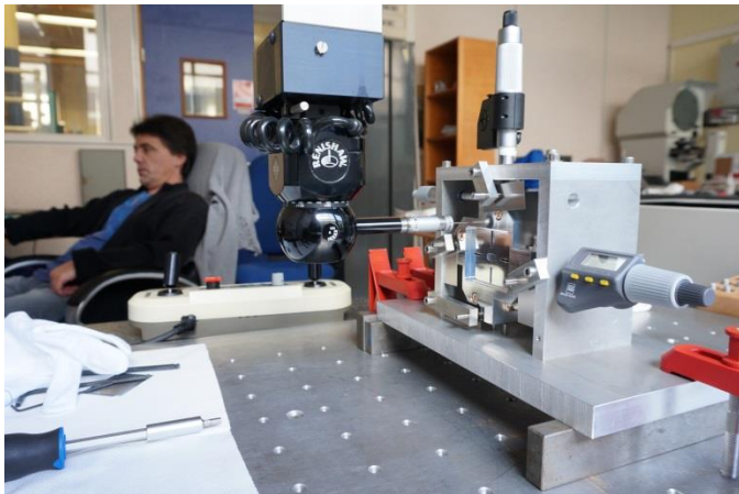
Adjustment bench for doublet BPM
