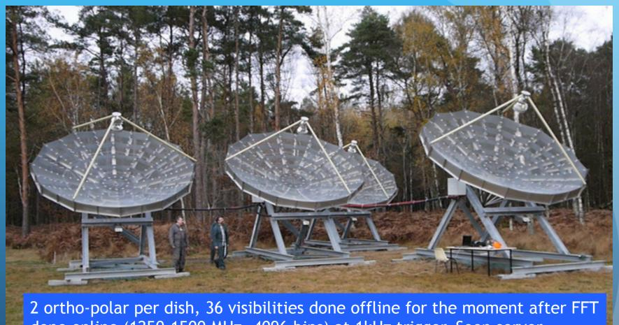
2 ortho-polar per dish, 36 visibilities done offline for the moment after FFT done online (1250-1500 MHz, 4096 bins) at 1kHz trigger. Soon server machines will compute the visibilities online.
