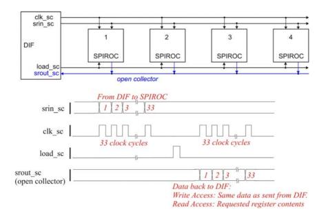
After a slow-control access, the addressed SPIROC sends back the data in additional 33 clock cycles to the DIF for verification, or for reading the requested data (read- or write access from DIF). In case of a write access, the SPIROC simply sends back the data it has received. The advantages of this setup are:
