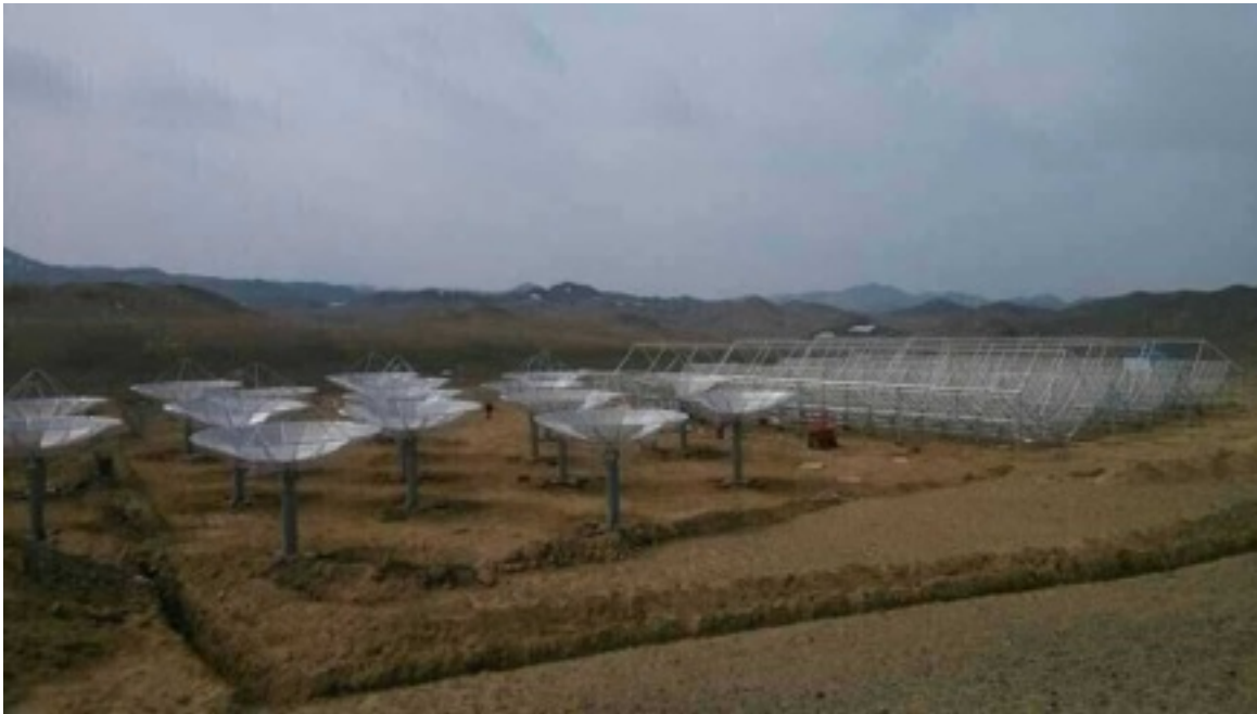
Photograph of Tianlai telescope from early April 2015. In view is a 3 cylinder array (the main part of the project) and part of a 16 dish array. A person can be seen in the distance for scale.
