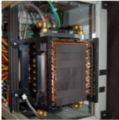
XPAD3 : 130 x 130 \mu\text{m}^2 pixels
