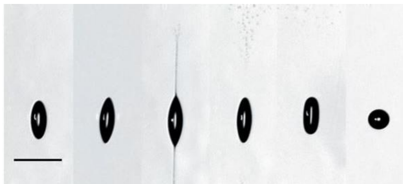
Instability of a droplet at the Rayleigh limit Denis Duft, and al.
