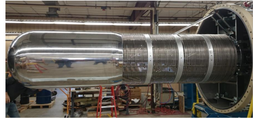
Pelletron Generator from NEC (ANDROMEDE Project)
