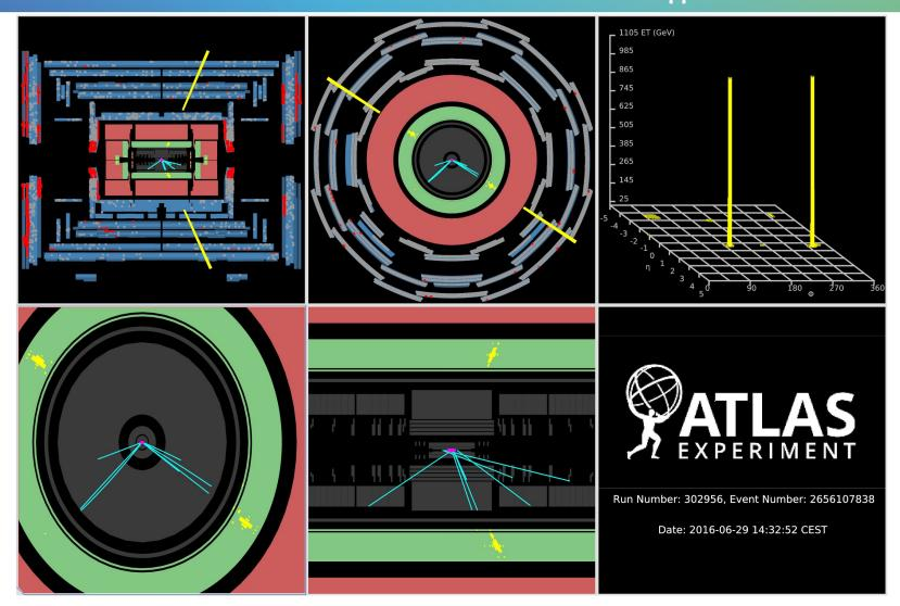
• **Leading photon:** unconverted,  $E_T = 1.1$  TeV,  $\eta = 0.45$ ,  $\varphi = -0.58$ ,  $E_T^{\text{iso}} = 5.2$  GeV
