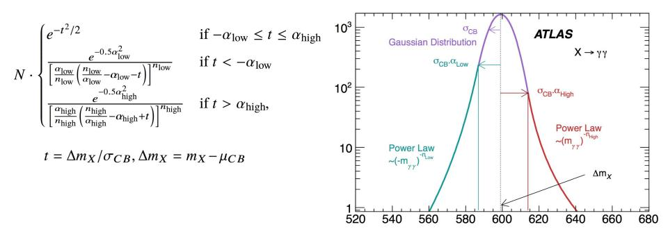
The parameters  $\mu_{CB}$ ,  $\sigma_{CB}$ ,  $\alpha_{low}$  and  $\alpha_{high}$  are parameterized as second order polynomials of the mass. The parameters of these second order polynomials are fitted with the values from the individual fits.
