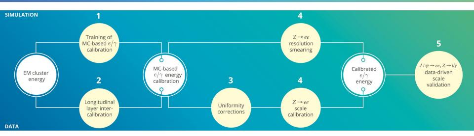
**1** - Optimisation of  $E_{rec}/E_{truth}$  using multivariate algorithm (MC-based)
