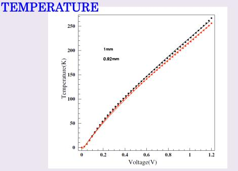
Simulation: mean temperature to which the fiber is heated as a function of the applied voltage (fiber reflector @2K)
