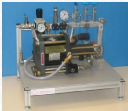
Compressor Compress up to 1000 bar
