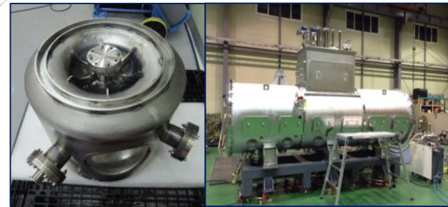
SSR SC Cavity and its Cryomodule
