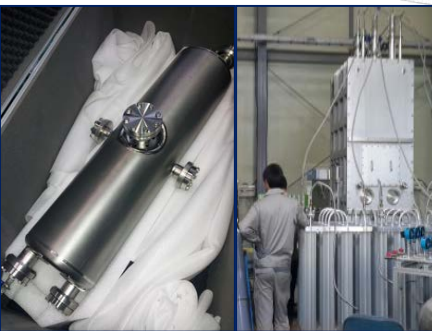
HWR SC Cavity & its Cryomodule
