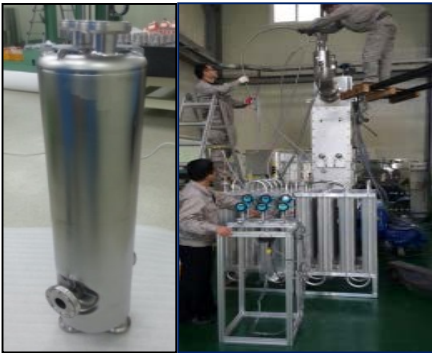
QWR SC Cavity & its Cryomodule
