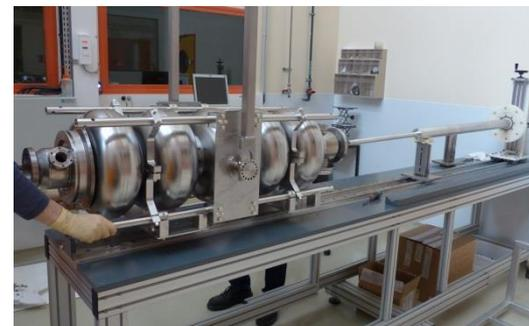
Cathode's insertion in horizontal position
