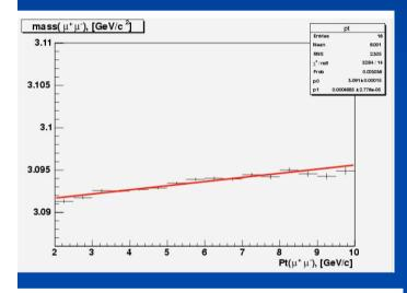
Standard material description still inadequate; photon conversion distribution indicates extra material to be z-dependent and in several locations
