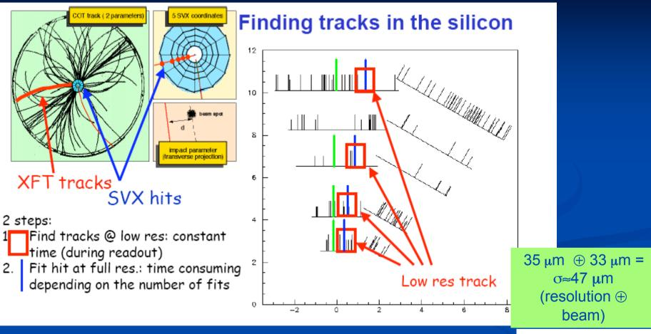
On-line tracking reconstruction allows design of specific triggers for heavy flavors; widely used in low-pt physics, extension to high-pt under way
