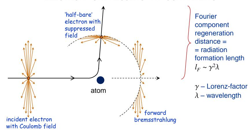
For photon energy  $\omega$  ~ 1 MeV and electron energy E ~ 10 GeV :  $l_F$  ~  $100~\mu{\rm m}$   $\gg$  electron mean free path
