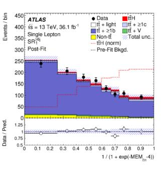
classify signal/background events based on other MVA outputs, kinematic properties of Higgs and top candidates, other event kinematic variables and discrete b-tagging information
