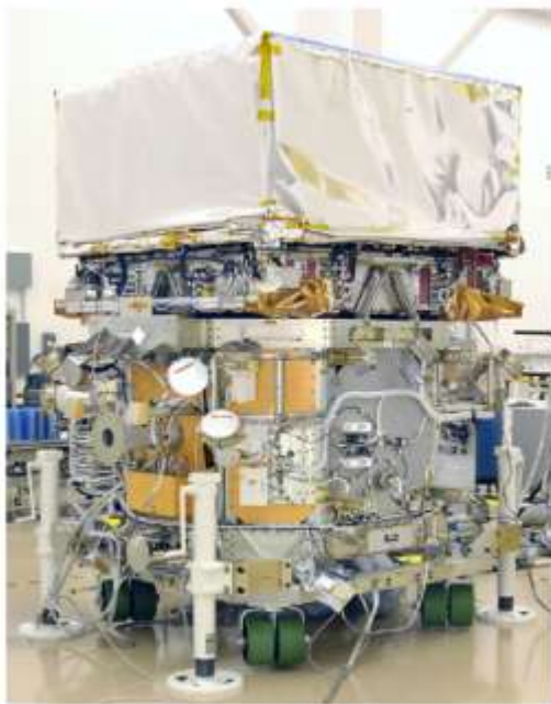
GLAST Observatory after the integration of the Large Area Space Telescope. Picture taken at the General Dynamic on December 2006.
