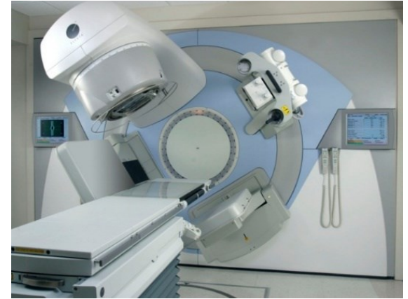
Clinical electron accelerator (X-rays ~6-25 MV)
