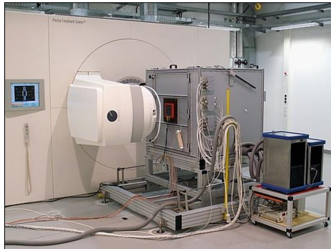
Water calorimeter in a clinical electron beam
