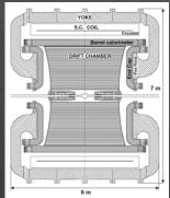
A unique volume, all stereo, cylindrical drift chamber, co-axial to B (0.6 T). Rin = 25 cm, Rout = 200 cm, L = 2.8÷3.3 m, 12+46 co-axial layers, at alternating sign stereo angles from 60 mrad to 150 mrad. Square cell size  $2x2/3\pi$  (inner 12) and  $3x\pi$  (outer 46) cm<sup>2</sup>. Total number of drift cells 12582. Total number of wires 52140
