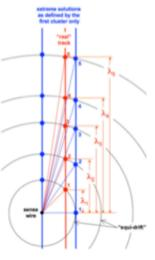
For any given first cluster (FC) drift time, the cluster timing technique exploits the drift time distribution of all successive clusters  $\{r_i^{\alpha}\}$  to determine the most probable impact parameter, thus reducing the bias and the average drift distance resolution with respect to those obtained from with the FC method alone.
