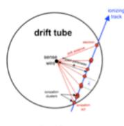
From the ordered sequence of the electrons arrival times, considering the average time separation between clusters and their time spread due to diffusion, reconstruct the most probable sequence of clusters drift times:  $\{t_i^a\}$   $i=1,N_a$
