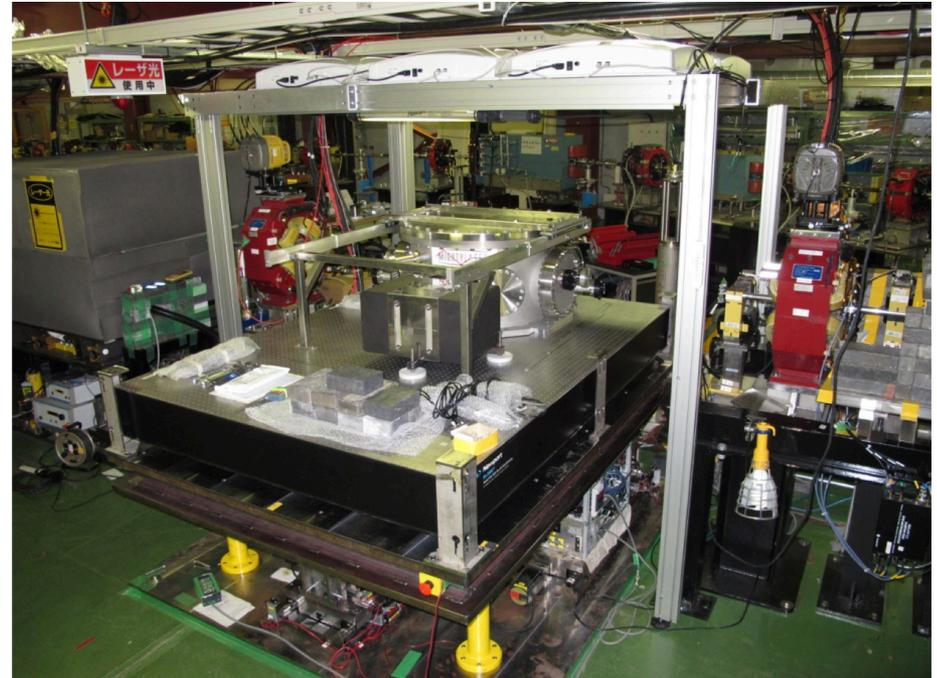
X-ray /  $\gamma$ -ray generation by laser-electron collision
