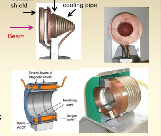
All the intensity monitors can be tested separately with the same test signal. A current generator and a distributor are controlled remotely to inject the current of test.
