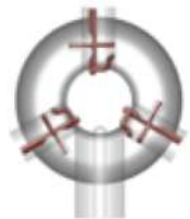
HOM 'Y' end-group with 3 coaxial couplers (here with scaled TESLA-type couplers)
