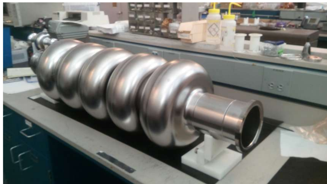
The first Nb 802 MHz 5-Cell cavity fabricated October 2017 at JLAB
