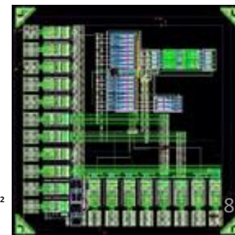
RD53: ROMIC: 1x1 mm 2 TSMC CMOS 65nm
