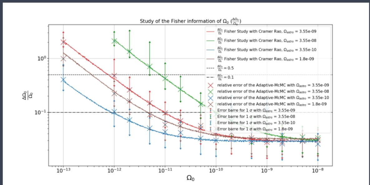
Uncertainty of the estimation of the Cosmological Amplitude from the Fisher Information study in line (with the Cramer-Rao calculation) and the parametric estimation from the A-MCMC in scatters for the channel A with the noise channel T. The upper horizontal dash line represent the error level 50%. In fact, above the line, the error is greater than 50%.
