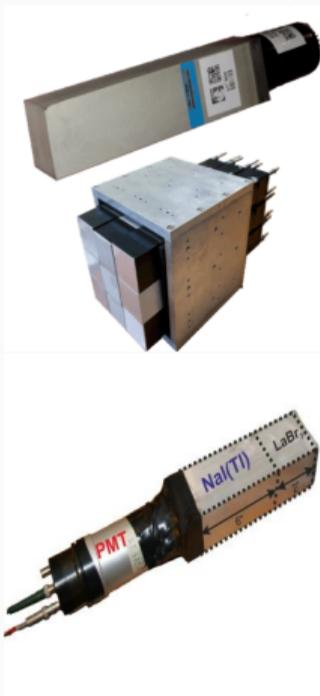
*Phoswich detector:* LaBr<sub>3</sub>/CeBr<sub>3</sub> crystal (2"x2"x2") + NaI crystal (2"x2"x6") + PMT
