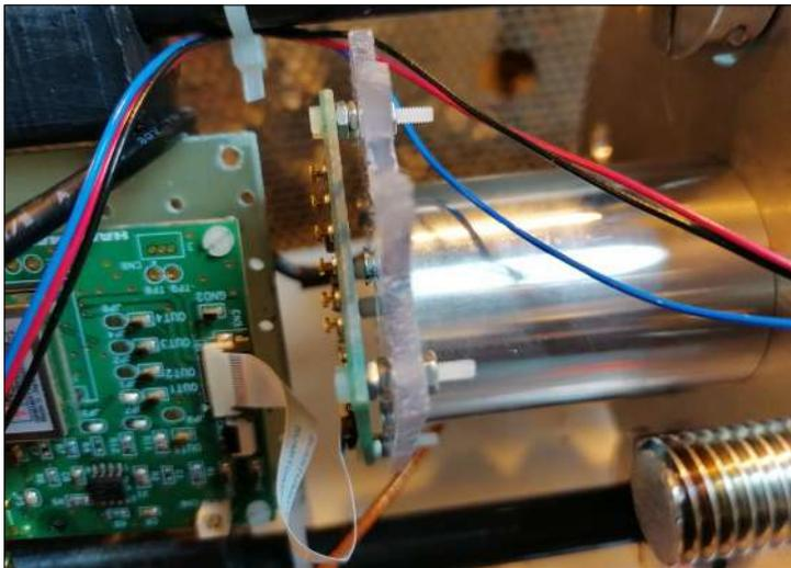
*Scintillator coupled to SiPM and connected to the driver circuit*
