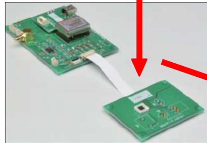
*SiPM connected to the driver circuit*
