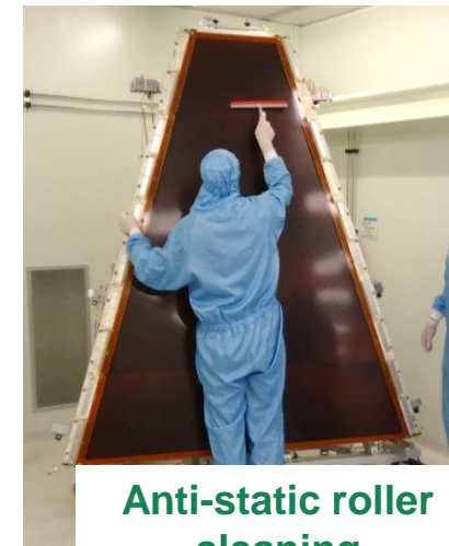
Anti-static roller cleaning (before passivation)
