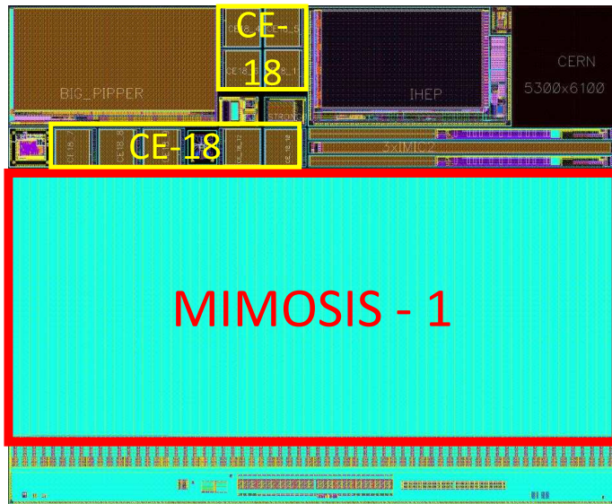
MIMOSIS-1 fabrication reticules
