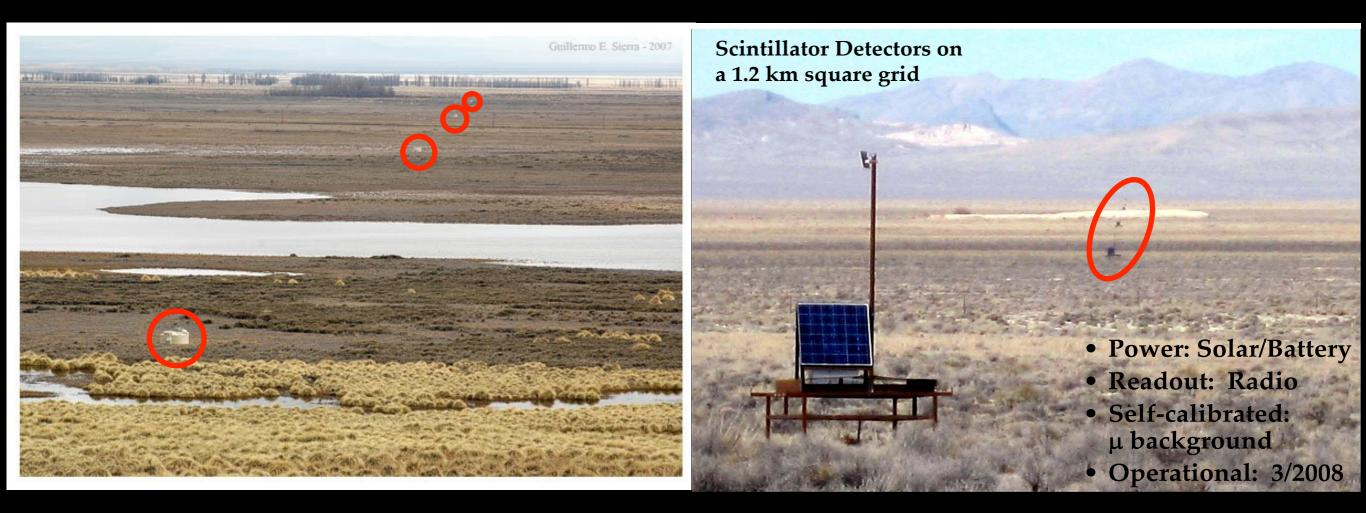
Perfectly aligned in the pampa, at a distance of 1.5 km one from another Perfectly aligned in the desert, at a distance of 1.2 km one from another
