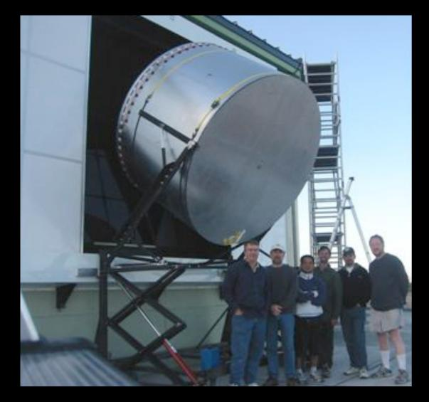
A CALIBRATED LARGE-DIAMETER, DRUM-SHAPED, LIGHT SOURCE PROVIDES AN ABSOLUTE, END-TO-END CALIBRATION
