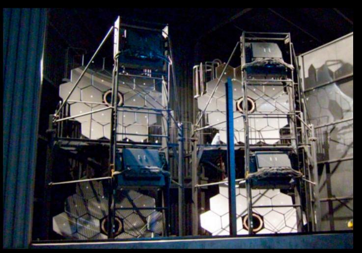
3 M SEGMENTED MIRROR 256 PMTS CAMERA 15° x 18° FOV
