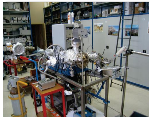
Setup for degazing rate measurement
