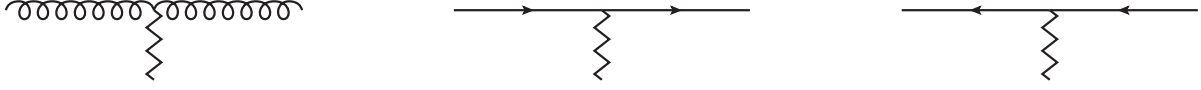
FIG. 5. Feynman diagrams relevant for the calculation of the LO impact factor describing the hadroproduction of a light jet. Zigzag lines stand for Reggeized gluons.
