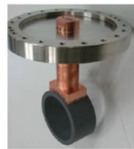
DESY inter-cryomodule beam line absorber for 100 W at 70 K temperature
