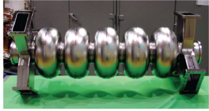
748.5 MHz JLab High Current ERL-FEL cavity prototype
