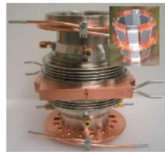
Cornell injector beam line absorber for up to 200 W at 80 K temperature
