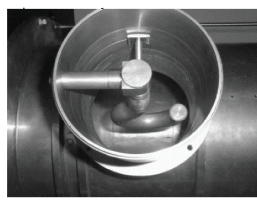
Soleil L-coupler for longitudinal modes
