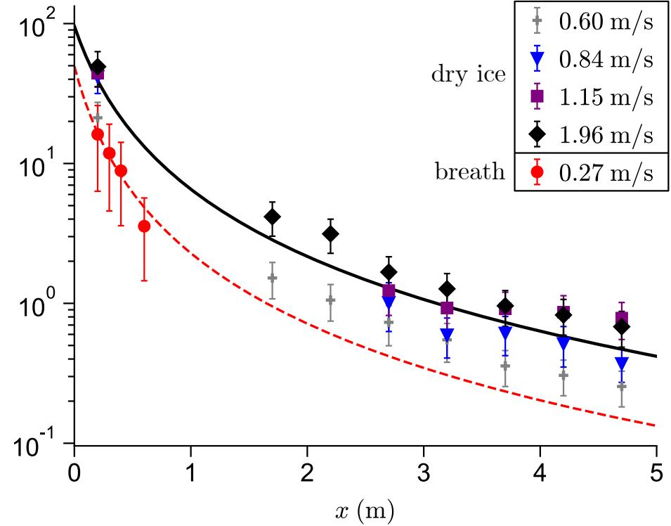
$$\frac{\rho_{\text{CO}_2} (\bar{C} - C_e) \bar{v}}{\dot{m}} = \frac{1}{\alpha^2 (a + x)^2}$$
