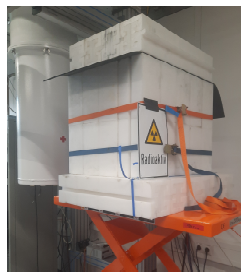
Portable thermal neutron source ( ^{252}\text{Cf} source in moderator) near a cryostat at TUM for the first CRAB experimental measurement
