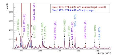
tag of fission events using <sup>235</sup>U diluted in liquid scintillator
