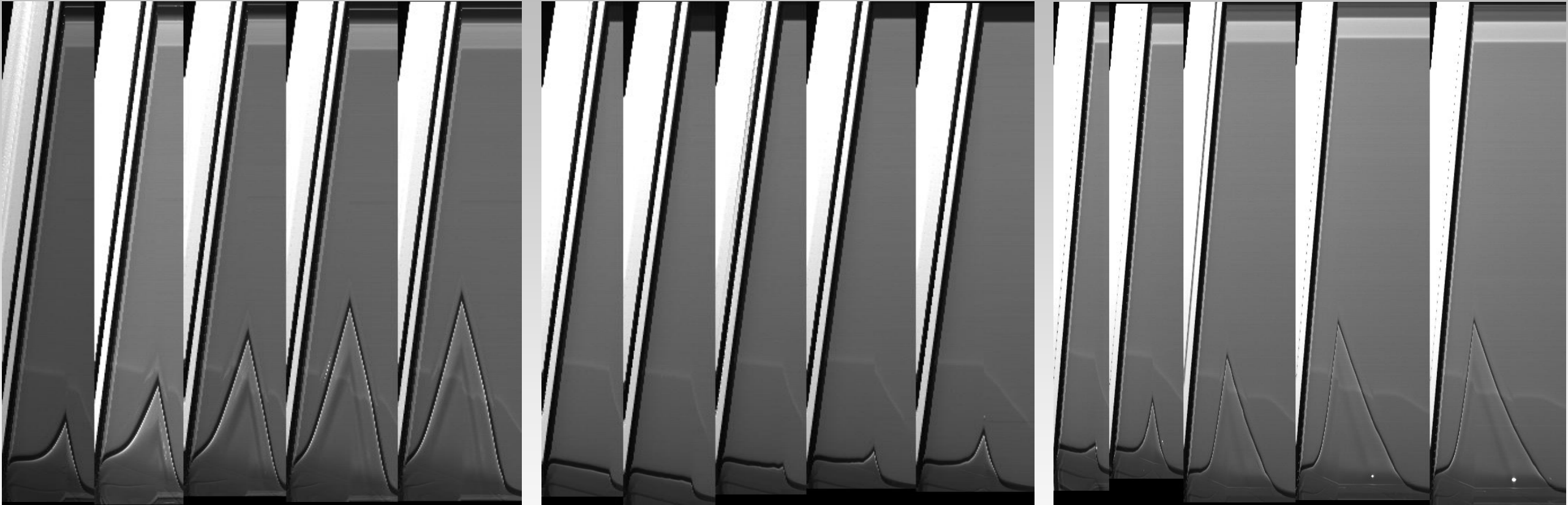
Figure 11 – Waiting time for Sylgard 527 between dipping of the substrate at Ca = 4 \cdot 10^{-2} . Left : Wait time = 30s. Middle : 100s. Right : 1000s.
