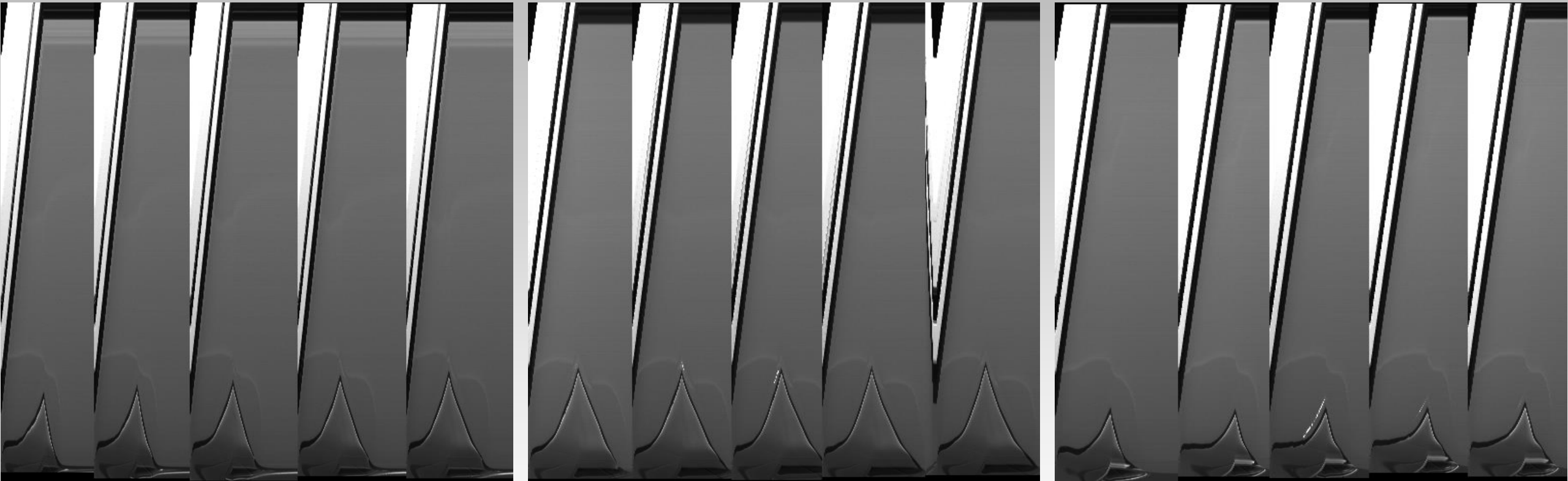
Figure 12 – Waiting time for Sylgard 184 between dipping of the substrate at Ca = 4 \cdot 10^{-2} . Left : Wait time = 30s. Middle : 100s. Right : 1000s.
