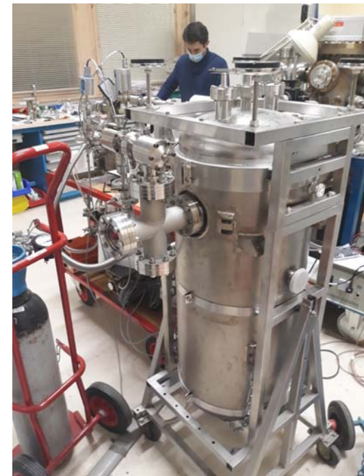
Plasma cleaning set-up with the SPIRAL2 cavity
